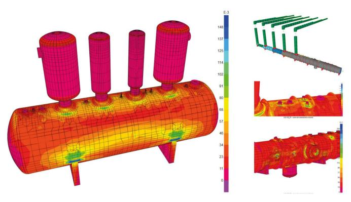
Calculation of piping and condensate tank for the air condenser, including determination of reactions and sizing of anchors to the foundation.
